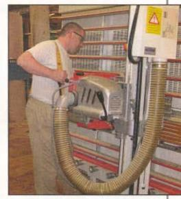
Accurate cuts — Matthew Malley uses a Striebig vertical panel saw for most of the cutting chores at H&B Woodworking in Plainville, CT. Malley is co-owner of the business and runs the shop.
