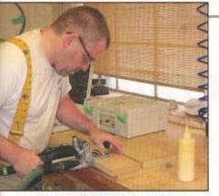
Speedy joinery — Malley likes the Festool Domino for fast, efficient and strong loose-tenon construction when he makes face frames and other joinery.
