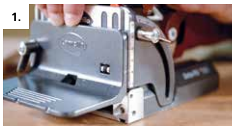
1. Locate the angle stop
