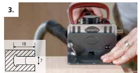
3. Mill a P system groove
