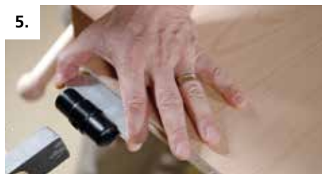
5. Tap in the fastening pins
