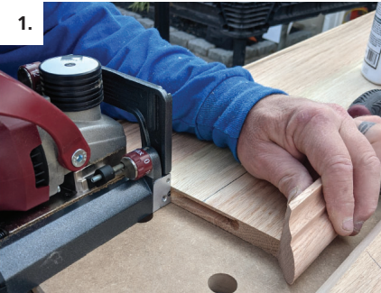
1. Make 14mm P-System slot in edge of tread and bullnose return
