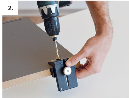
2. Drill 6mm access hole in bottom of tread for male Clamex connector, using drill jig
