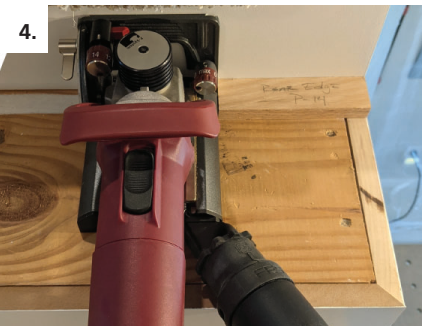
4. Create stop block to reference P-System slot in riser
