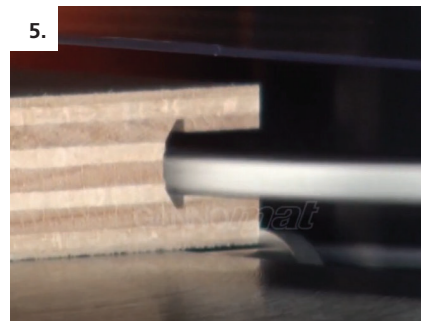
View from inside the Gannomat machine as it mills the P-System slots and Clamex access holes
