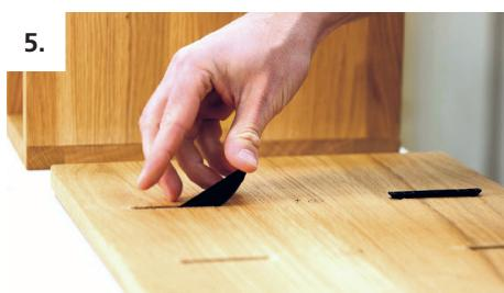
Insert the Tenso P-14 element into the P-10 grooves.
