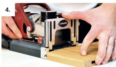
Mill the P-System groove on the front side with depth setting 18.
