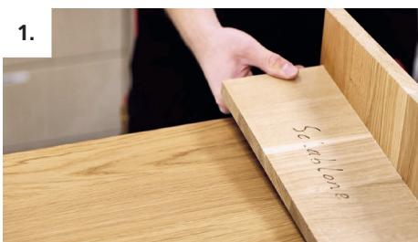
Use a template with uniform spacing instead of marking repeatedly.
