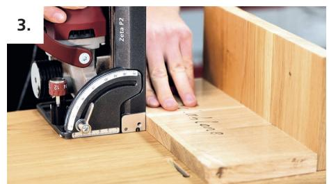
Perform milling on the surface on both sides with depth setting 10.
