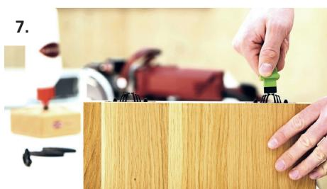
Preload the Tenso P-14 to facilitate assembly.
