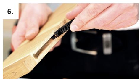
Insert the Tenso P-14 element into the P-18 groove.
