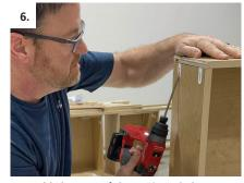
Assemble bottom of drawer into dado first and put side of drawer on next. Turn the clutch down on drill drivers. Using an impact driver is not advised!
