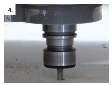
Rout or drill the Cabineo pocket to correct depth and rout additional shoulder for flush-mount installation.
