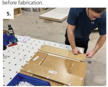
Install Cabineo connectors into pockets. Use mallet if necessary.
