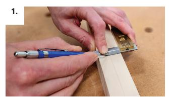
Lay out connector slot location on back side of face frames
