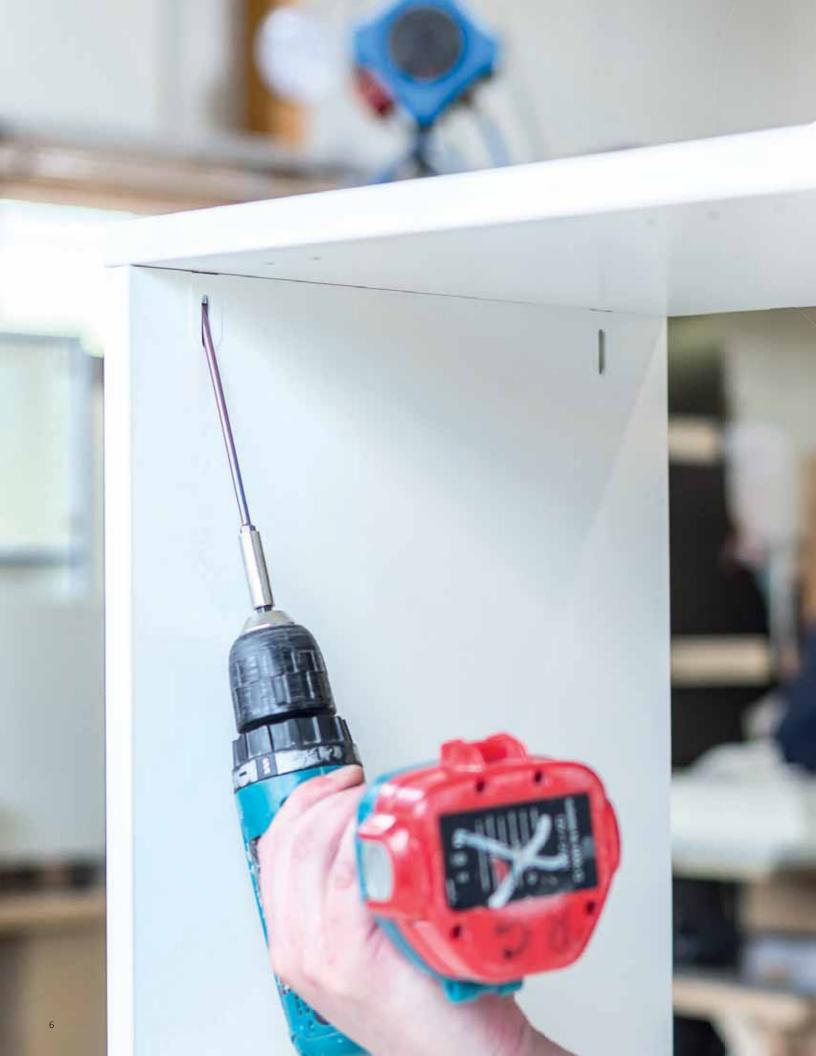
With the protruding screw the workpieces are perfectly aligned. Then we simply join them with a cordless drill. >>
