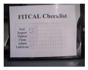
A FITCAL checklist (shown above) records the six key preventive maintenance operations every grinding shop should perform: FEEL, INSPECT, TIGHTEN, CLEAN, ADJUST, LUBRICATE
