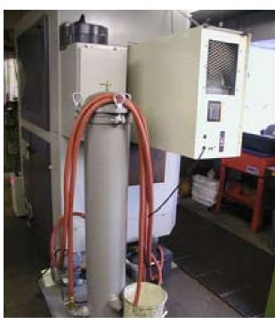
Needham Saw is running oil coolant on the UniMAX. This optional coolant filtration system, offered by Colonial Saw, eliminates the need to clean the coolant tank and change out the oil.
