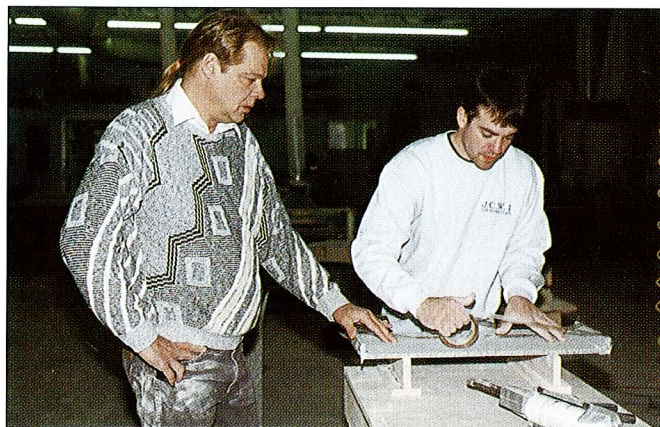
(top) Coming off the saw, the two sides of the V-groove are held together by tape that was applied to the face side of the solid surface material before grooving. Adhesive is then applied to the groove.
