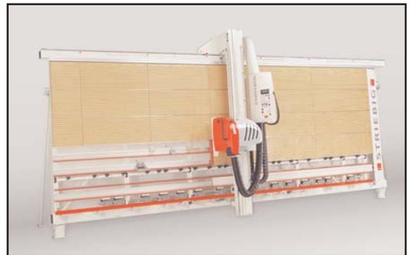
Many Striebig models are now available with performance-enhancing options such as digital measuring, split-blade scoring, programmable electronic positioning, angle cutting, dado cutting, V-grooving, and a two-speed motor. Striebig’s TRK dust-extraction system keeps dust to an absolute minimum, and a new vacuum system allows bottom-edge trimming without flipping the panel.
