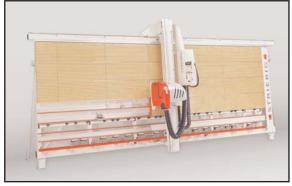
electronic positioning, angle cutting, dado cutting, V-grooving, and a two-speed motor. Striebig's TRK dust-extraction system keeps dust to an absolute minimum, and a new vacuum system allows bottomedge trimming without flipping the panel.
