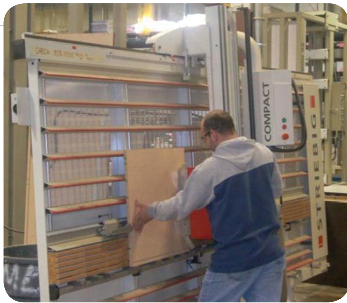
Vertical panel saws have made material handling much easier for Metropolitan Cabinet & Countertops
