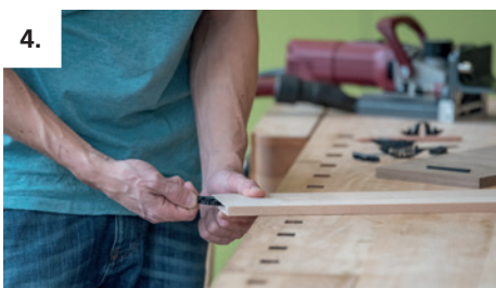
Inserting a half shell with a spring into the drawer sides
