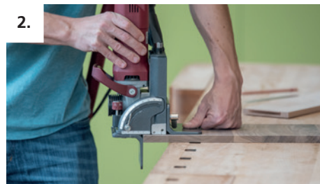
Cutting a profile groove into the front piece using a 10 depth setting
