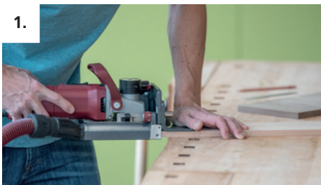
Cutting a profile groove into the side using an 18 depth setting
