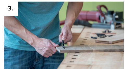
Inserting a half shell without a spring into the front piece
