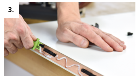
3. Preload connector and apply adhesive
