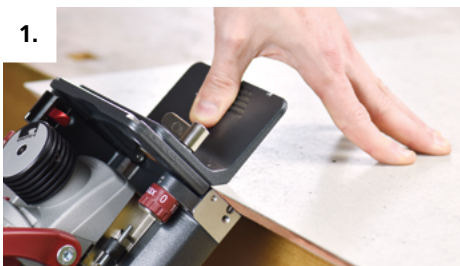
1. Mill P-System grooves with depth setting 10 into the cutting surfaces
