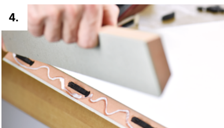
4. Join together workpieces and wait until adhesive has hardened
