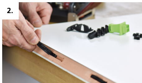
2. Insert TensoP-10 connector half into the workpieces
