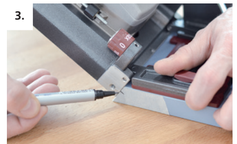
3. Transfer the centre of the milling to the workpiece
