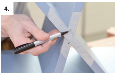
4. Hold workpieces together and transfer marking
