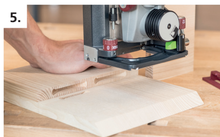
5. Cut groove into the surface
