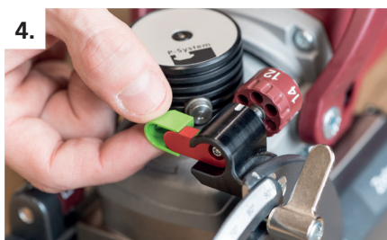
4. Attach the P-System depth adjuster cap 4 mm for P-8 (groove depth 8 mm)
