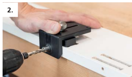
2. Drill a 6 mm access hole in to the edge using the P-System drill jig
